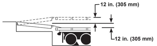
The XL hydraulic dock leveler is designed to compensate for a maximum  $\pm 12$  in.\* (305 mm) of height difference between the loading dock and the transport vehicles bed. DO NOT use the dock leveler if the transport vehicles bed is more than 12 in. (305 mm) higher or lower than the dock floor.
