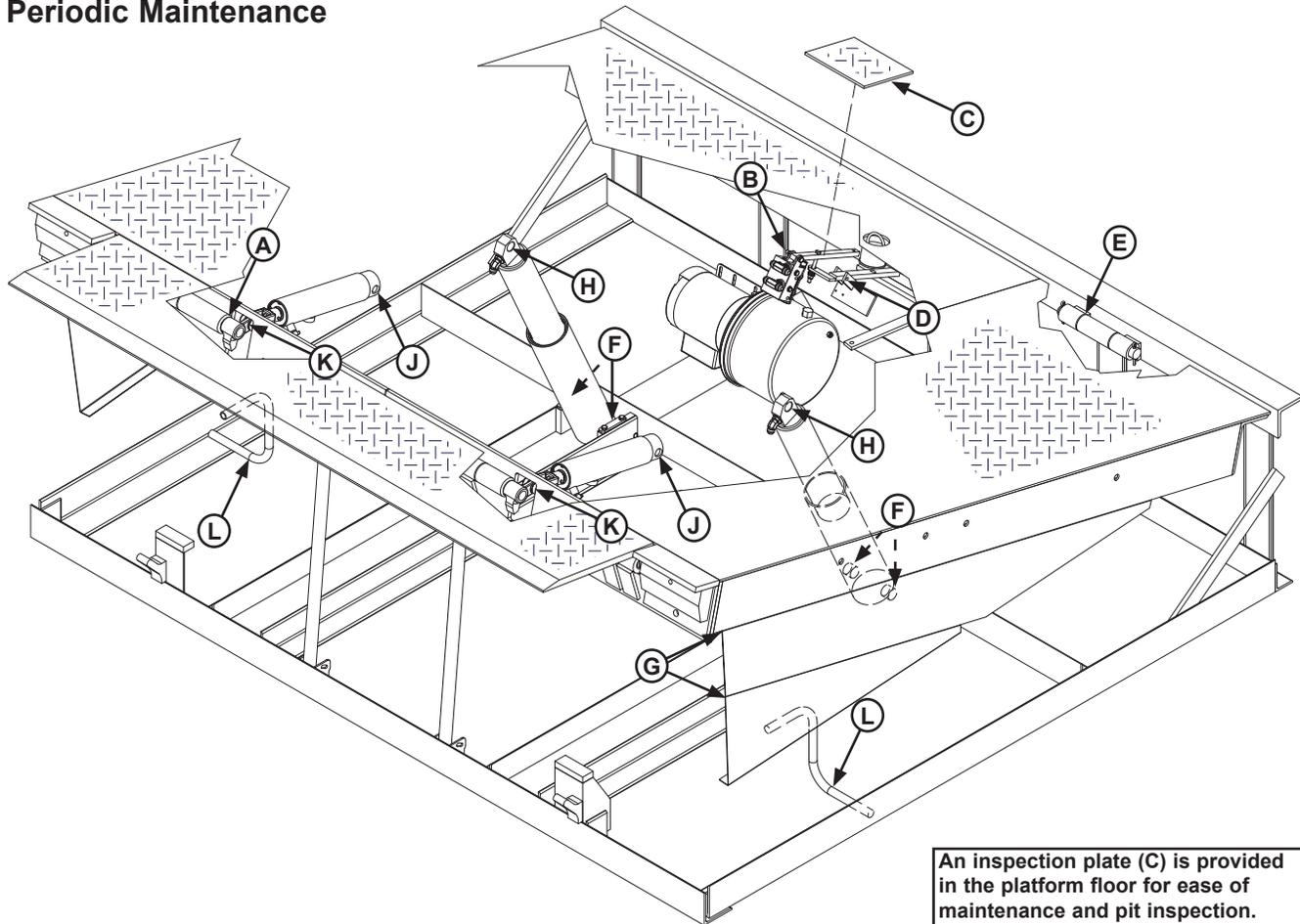
An inspection plate (C) is provided in the platform floor for ease of maintenance and pit inspection.
